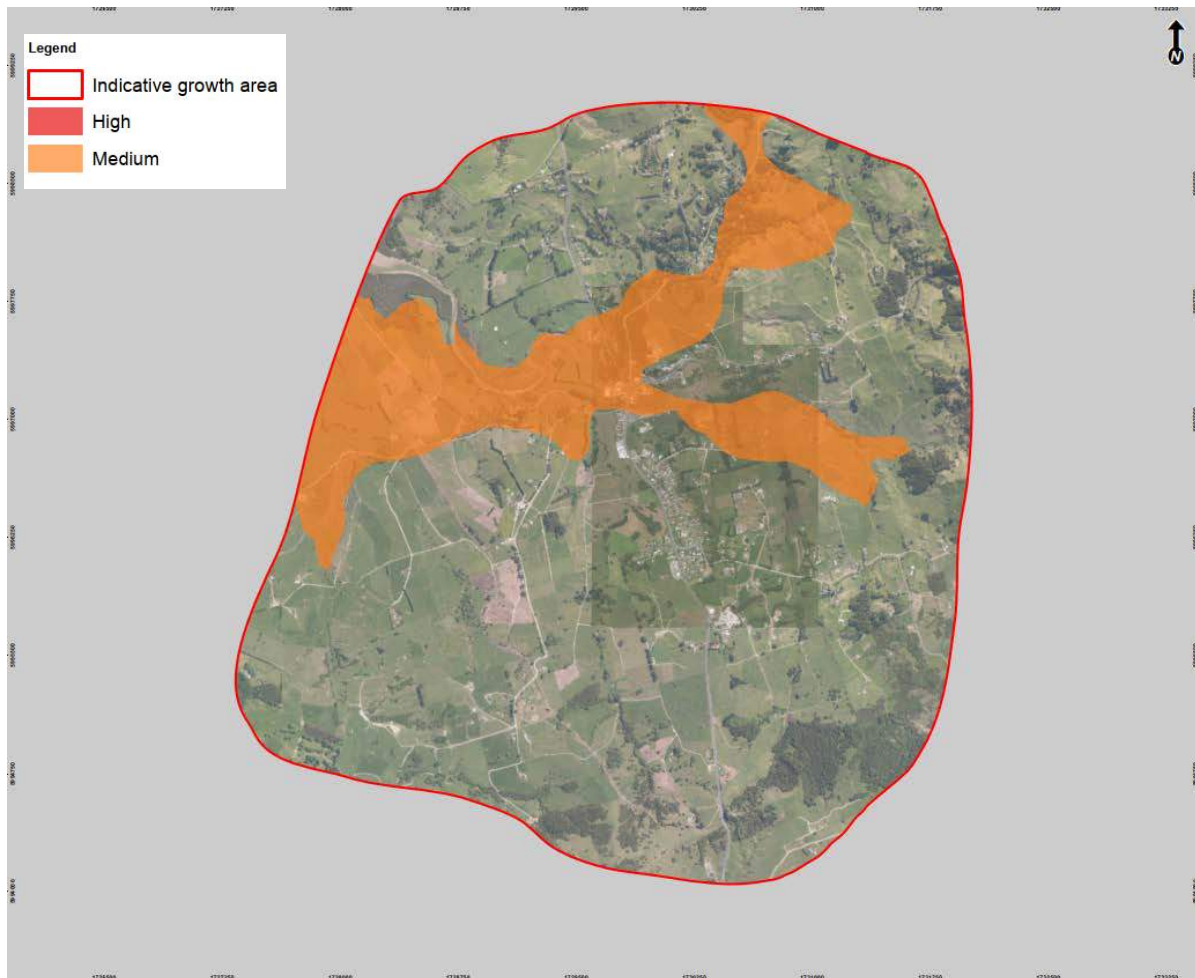
Figure 7: Liquefaction and Lateral Spread Susceptibility Plan
